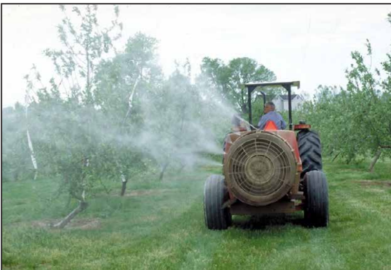
SPRAYING AN APPLE ORCHARD WITH AN AIR-BLAST SPRAYER. (PHOTO: JOHN HARTMAN, UK)
