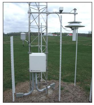
A KENTUCKY MESONET WEATHER STATION. THIS NETWORK OF AUTOTMATED WEATHER AND CLIMATE MONITORING STATIONS WAS DEVELOPED BY WESTERN KENTUCKY UNIVERSITY.
