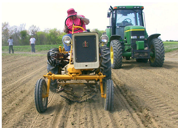
Figure 3-4-A. A Buddingham weeding machine being used to place soil around the crowns of newly planted strawberry plants.
