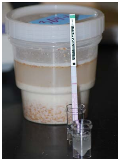
Figure 3. A corn sample being tested for mycotoxins using supplies from a test kit.
