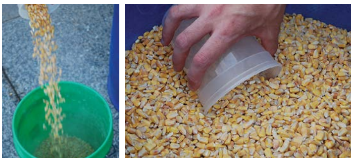
Figure 1. Several subsamples of corn are pooled to form a larger representative sample.
